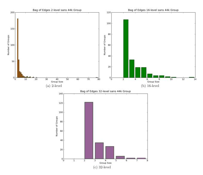
Figure 7: Working sets with the bag-of-edges algorithm. Higher levels result in much smaller groupings.
