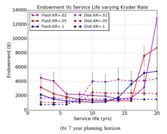
Fig. 2. As  $K_r$  slows down we need longer lived devices to keep the long-term storage costs low.
